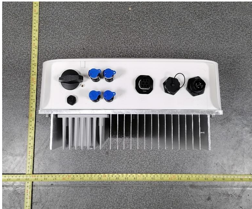
Figura 3, Vista do painel de terminais Figure 3, Terminal panel view
